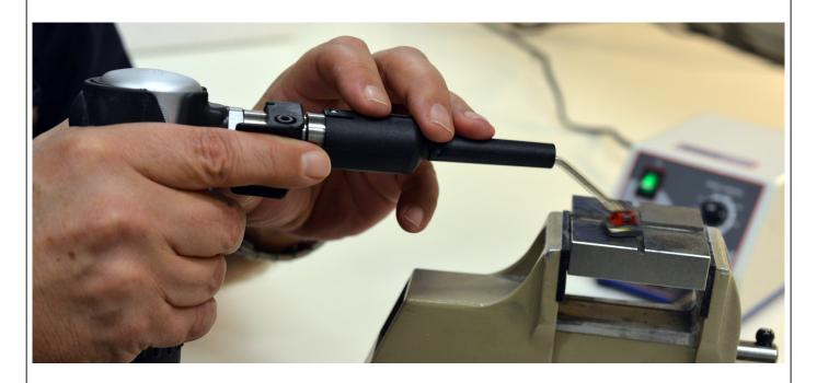
The Classic polishing/filing machines, which have been the preferred choice for tool and mould-makers for more than 60 years, incorporate a comfortable tool-holder to improve ergonomics and flexibility.
